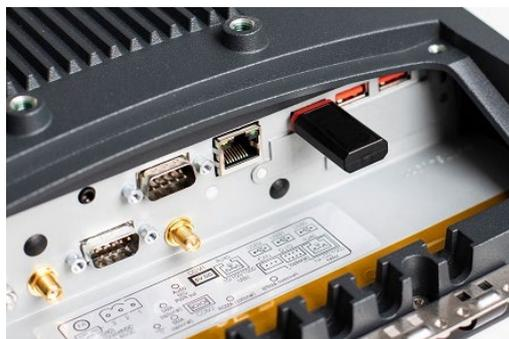
Figure 3.1: DLT-SA6100 Sensor Stick connected to ADLoG VMT
