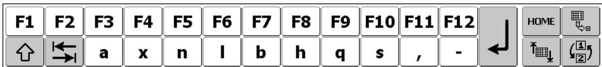
Figure 5.2: Software keyboard with terminal emulation keyboard layout
