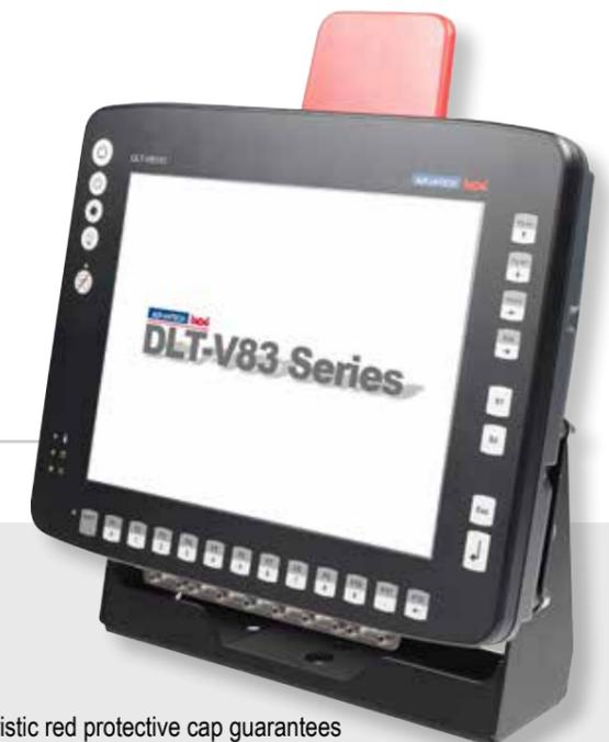
The characteristic red protective cap guarantees high mechanical stability and protects the antennas from being damaged. This guarantees a stable WLAN connection, even in difficult conditions. In addition, these terminal antennas support both frequencies used by WLAN, 2.4 and 5 GHz, as well as the WLAN standard 802.11n.
